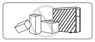
1.4.4. Do not put anything into the inlet or outlet, and do not remove the fan cover and the running fan to avoid injury.
