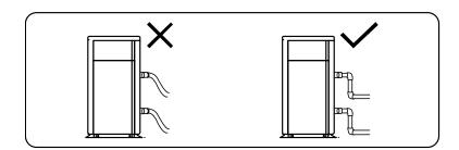
2.1.2. In order to guarantee the heating efficiency, the water pipe length should be ≤10m between the pool and the heat pump.
