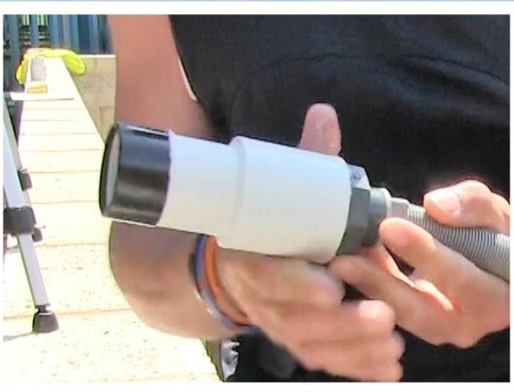
Glue a 50mm slip adaptor on the end of the piece of pipe you have just cut.
