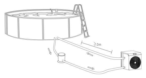
Note: Do not install the unit in a confined or insufficient ventilation location, or in a location where it may block the air intake. These locations can affect the flow air c. It will cause the air to recirculate, resulting in reduced efficiency. It even may stop the system from running.
