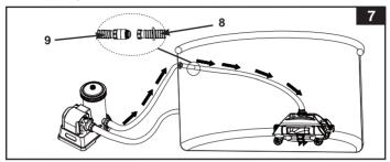
9. Turn on the filter pump, and make sure water is flowing through the auto cleaner. The auto cleaner is now moving and vacuuming the pool floor. See Fig. 8.
