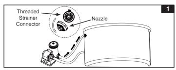
2. Screw the end of hose A (8) with adaptor to the threaded strainer connector, from inside of the pool. See Fig. 2.
