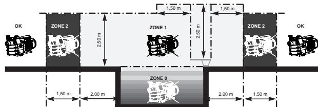
Install the pump in a dry, well-ventilated place. The motor requires the air to circulate freely around it to allow natural ventilation. Clear a space of at least 0.5m around the pump. Check regularly that no objects, leaves or other debris are blocking the motor cooling system.
