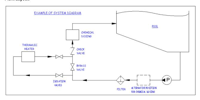
Chemical dosing systems should not be installed adjacent to the heater. If installed upstream of the heater it must be before the filter. If installed downstream, a check valve must be fitted to prevent backflow of chemicals when the filter pump is not operating. There should be a drop in level between the pipe leaving the heater and entering the dosing system.
