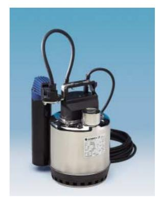
This float switch allows the pump to be used where standard float design cannot work due to insufficient space. The pump with this system can only be installed vertically and can only be used with clean water.
