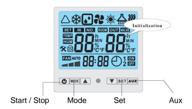
3. After a few seconds the display shows ROOM and a temperature. This is the temperature of the air surrounding the heat pump.
