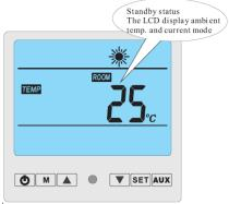
2. Press the set button repeatedly until SET NO 01 shows with the set point temperature in degrees C.
